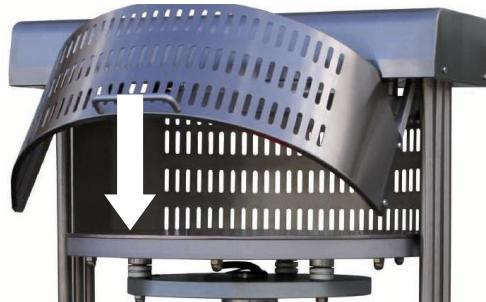
**⚠ If the first start the bottom plate is not lifted completely, but rises only about 2 cm, the phase sequence is not correct.**
